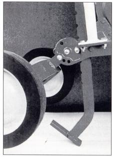
Wheel assembly lifts up and locks out of the way. Clevis pins hold wheel assembly to rear hitch. Wheels lock in four positions and are easily removed when both outer pin and center pin are withdrawn. Notches on rear skid allow depth adjustment. Skid is secured by same pin/clip setup.
