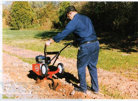
The tines on some tillers are set back farther than standard front-tine tillers, which position more of the engine weight directly over the tines for greater digging capacity.
